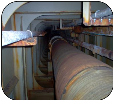
Badly corroded ballast pipe manually prepared and filled using 302 Epoxy Repair Cement, 30mtr length of pipe then encapsulated using 301 Epoxy Resin and Hardener and Glass Tape
