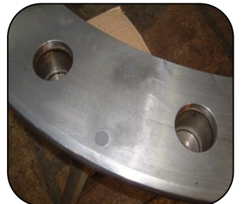
Turbine cover repaired using 107 Metal Repair Paste XL (Egypt)
