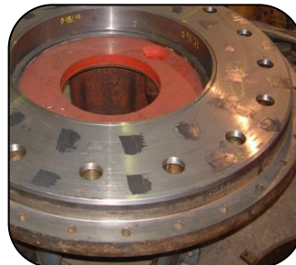
Turbine cover repaired using 107 Metal Repair Paste XL (Egypt)
