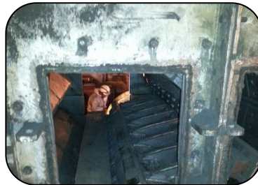
Coal grinder at a steelworks relined and repaired using 204 Heavy Duty Ceramic Repair Paste
