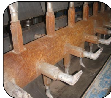
Process equipment abrasive blast cleaned and resurfaced using 202 Ceramic Repair Fluid
