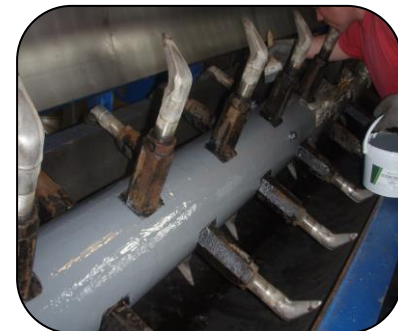
Process equipment abrasive blast cleaned and resurfaced using 202 Ceramic Repair Fluid
