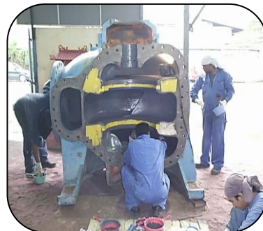
Split case pump rebuilt and protected using 201 Ceramic Repair Paste and 202 Ceramic Repair Fluid
