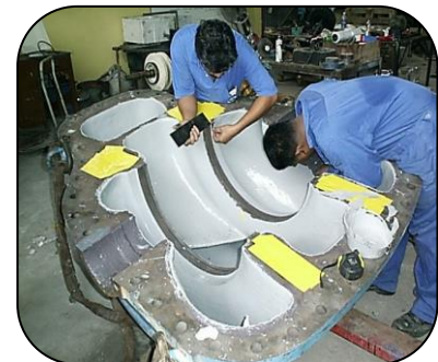
Split case pump rebuilt and protected using 201 Ceramic Repair Paste and 202 Ceramic Repair Fluid
