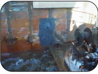
Holed ship hull repaired in sub-zero temperatures using 106 Metal Repair Paste XF and a formed steel plate
