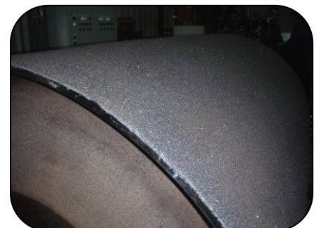
Belt rollers resurfaced using 102 Metal Repair Fluid and Aluminium Oxide
