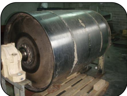
Belt rollers resurfaced using 102 Metal Repair Fluid and Aluminium Oxide
