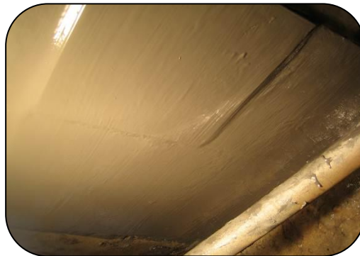
Belt rollers resurfaced using 102 Metal Repair Fluid and Aluminium Oxide
